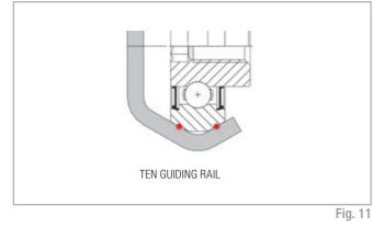
The two inclined bearing slopes run on the two slopes of the V-shaped raceways of the TEN rail. These 2 points contact on each roller in upper or lower raceway, assure both radial and axial load capacity.
