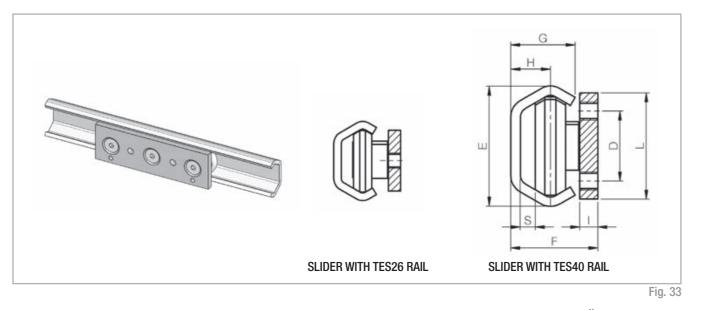
The sliders CES26 for the rail TES26 feature a zinc plated steel body with two fixing holes. With the rails TES40 can be used the sliders CEN40-135 indicated on page XR-10 that have a body with black color surface treatment.
